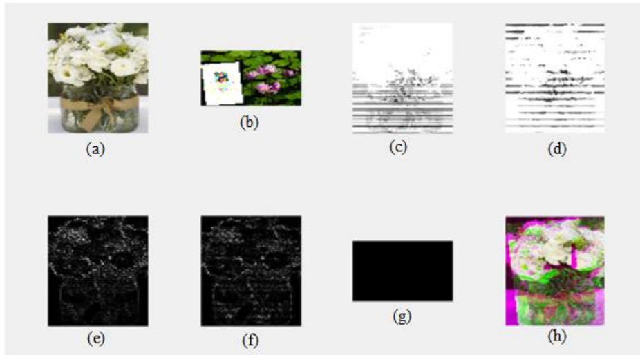
Fig. 7: (a) original, (b) stego (c) LL, (d) LH, (e) HL, (f) HH of encrypted, (g) watermarked image, and (h) decrypted image for DWT based technique.
