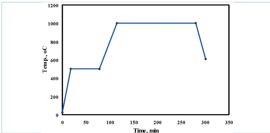
**Fig. 1: Sintering cycle for Cu/WC-TiC-Co/graphene nano palettes composite.**
